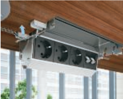
Preparing Deskbox fastening The fastening hole strips located on the Deskbox are bent over the fixing rail contained in the scope of delivery.
