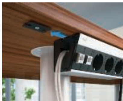
Mounting of the Deskbox on the fastening set, under-table mounting Push the Deskbox onto the fastening element from the side. The design panel must be removed in advance.
