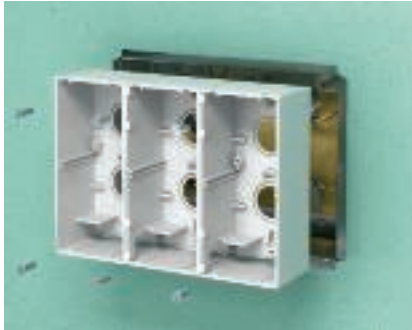
Housing mounting Insert the prepared housing base into the cavity wall support and connect the rear panel with the supplied fastening screws.
