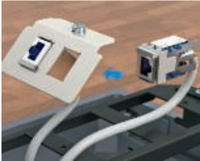
Mounting of Snap-In fastening frame Attach the Snap-In fastening frame to the connection module from the front and lock it in place. The Snap-In fastening frame allows the installation of the data technology modules in underfloor systems using a mounting support or support plate with a mounting opening 19.3 x 14.8 mm (Type C).
