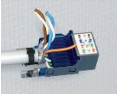
Device connection – cable sorting Attach the individual wires according to the connection table and fix them using the contacting terminal.
